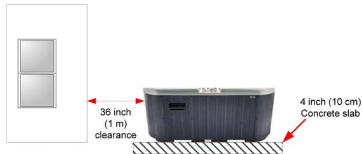
Figure 1 – Clearances and Support
