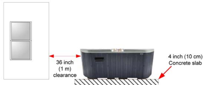
Figure 1 – Clearances and Support
